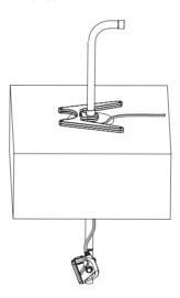
**10** Rotate the handle to aim the transducer.
