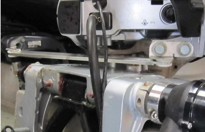
Steering Actuator Connected to Linkage
