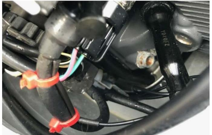
RPM Cable Installation
