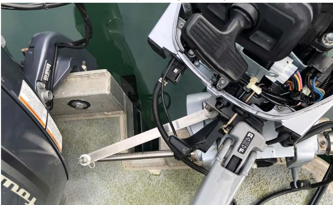
Top View of Steering Actuator
