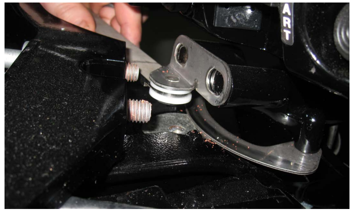
Installing the Steering Actuator Bracket Between the Tiller Arm and Motor
