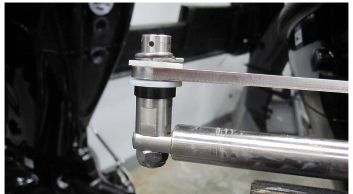
Steering Actuator Spacer Stack Order
