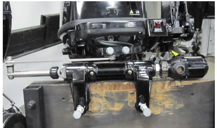
Complete Steering Actuator Installation
