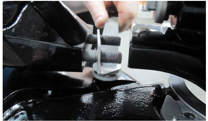
Installing the Steering Actuator Bracket Between the Tiller Arm and Motor
