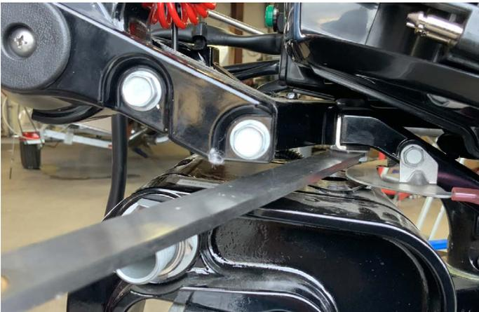
Motor Bracket Installed on the Motor
