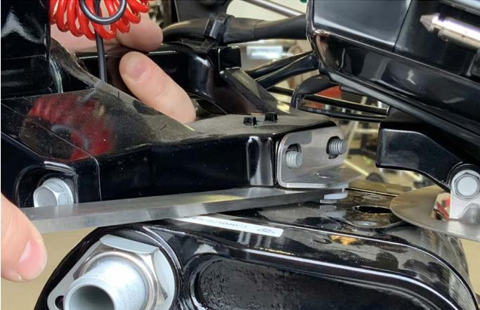
Installing the Motor Bracket Between the Motor and the Tiller Handle
