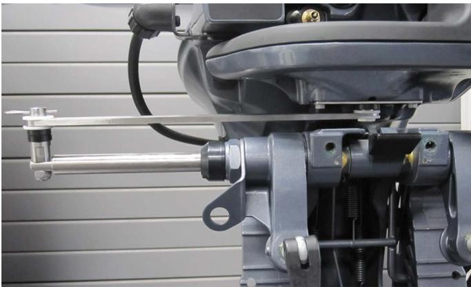
Complete Steering Actuator Installation
