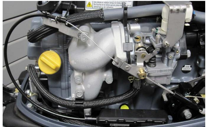
Throttle Actuator Installed on Yamaha Throttle Shaft
