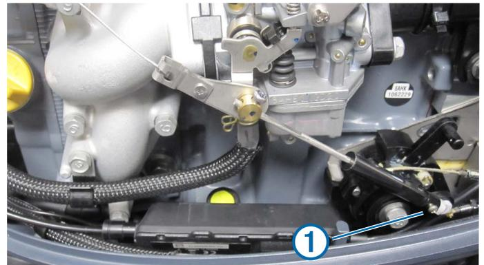
Barrel Slider Throttle Linkage
