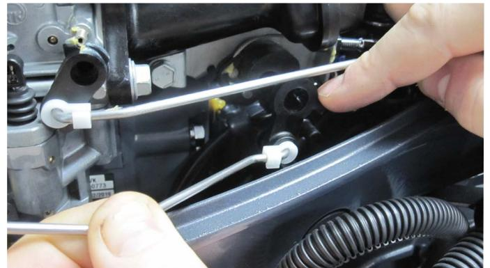
Bell Crank Lever Installed on Throttle Linkage
