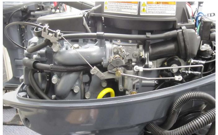
Throttle Actuator Installed on Yamaha Throttle Shaft
