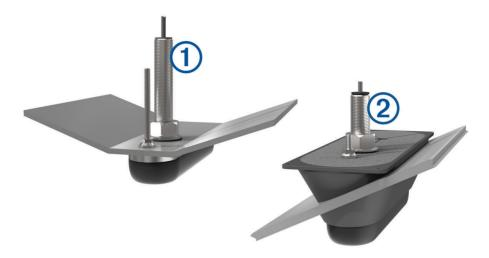
Optimal placement is parallel with the waterline.
