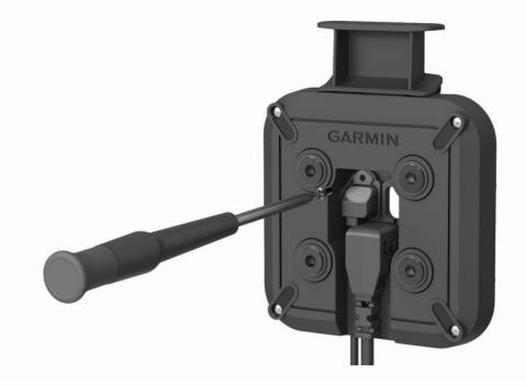
10 Replace the mount on the ball plate, and secure the mount using the 4 existing screws, washers, and nuts.11 Connect the External Iridium Antenna cable to the External Iridium Antenna connector on the mount.
