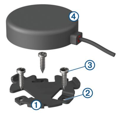
**2** Drill the three 3.2 mm (1/8 in.) pilot holes (optional).
