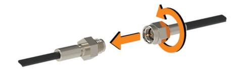
**12** Tighten the collar around the connected cables.
