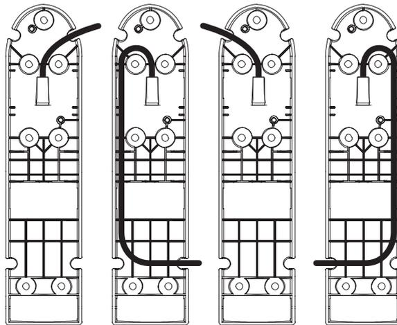
You must avoid pinching the cable or bending it too tightly.
