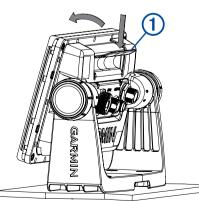
2 Tilt the device forward, and lift it out of the cradle.
