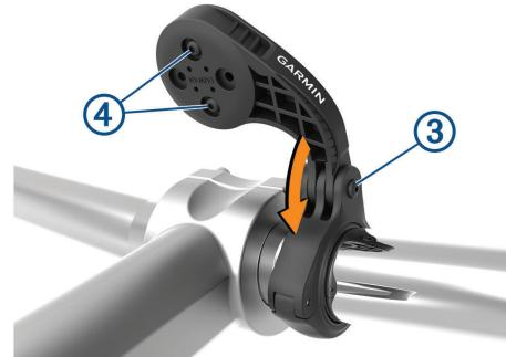
**6** If necessary, use the 2 mm hex key to remove the two screws on the back side of the mount **④**, remove and rotate the connector, and replace the screws to change the orientation of the mount.
