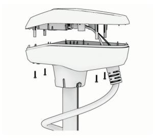
2 Carefully lift up the lid of the shaft cap to access the cable connectors inside.
