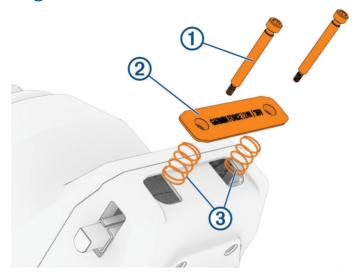
**NOTE:** The latch spring cover is under spring tension. Take care that you do not lose the cover and springs 3 during disassembly.
