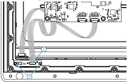
2 Remove the two screws 2 securing the power button board to the front case assembly.
