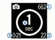
The device takes a series of photos at the selected interval. The screen displays the remaining number of photos the device can take ①, the number of photos the device has taken ②, the elapsed time ③, and the time in seconds until the next photo is taken ④.
