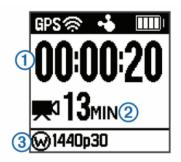
The screen displays the elapsed recording time ①, available recording time ②, and video mode ③.
