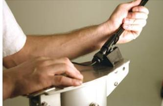
5. Tighten the lock nut by hand only (do not use any tool)
