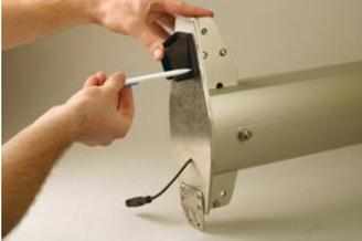
2. Drill the three mounting holes using a 3,2mm drill
