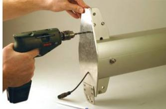
3. Mount the bracket with the three supplied screws
