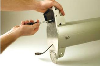
4. Insert the transducer into the bracket from front to back
